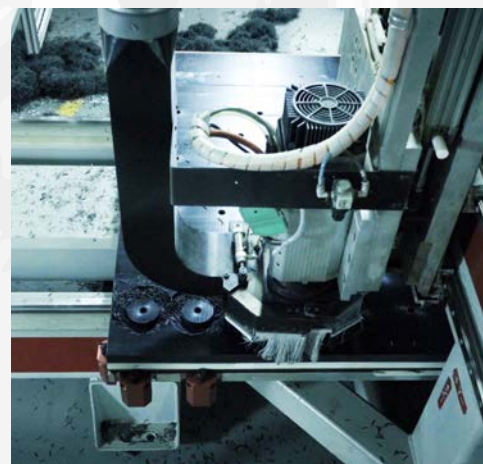
Up to 120" x 60" x 5" work piece at a max 22,000 RPM.
